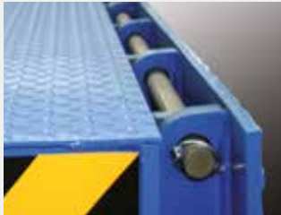
Lip axles and hinges: electrolytic bichromate to prevent corrosion. Self-cleaning hinges (Axle Ø29 mm.)
