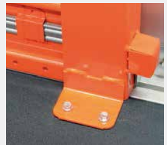
Reinforcement with anchoring to the ground.
