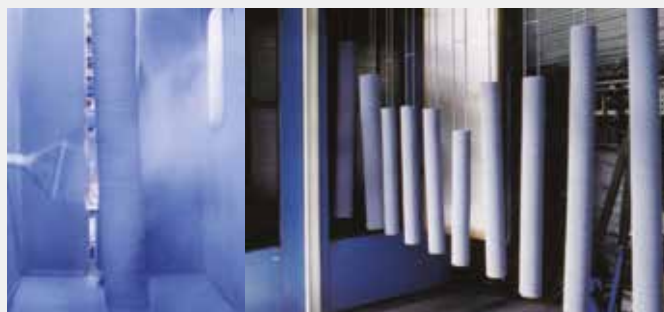
"Bombarding" installation of particles and powder paint.
